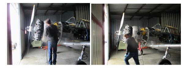
OK, here we go on installing the "muff"......here's Charlie starting the Dzus fasteners while I'm gathering all the nuts, bolts & washers for the forward mounts Now, all this is happening when a HUGE rain squall comes over the airport and is dumping 5000 inches of rain on us. The lights in the hangar don't work, so we have to open the doors to see what we're doing, which allows all the water to come blowing in....ya gotta be tough to to be an airplane mech!
